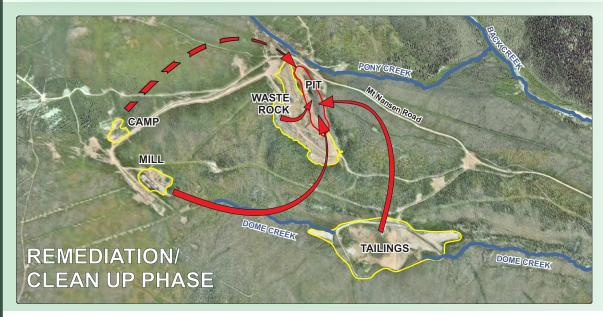
Mine tailings, waste rock and other waste material will be placed in the open pit and covered with an engineered barrier liner system.
